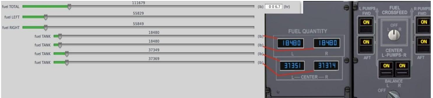
Above are the the main fuel controls. The left tank switches turn the fuel pumps on/off for the left wing tank. The right tank switches turn the fuel pumps in the right wing on/off. The center tank is controlled by the lower switches. The FUEL CROSSFEED switch allows the right engine to use fuel from the left tank and visa versa. The BALANCE switch will transfer fuel from the left tanks to the right tanks and visa versa if the aircraft needs to be balanced.
