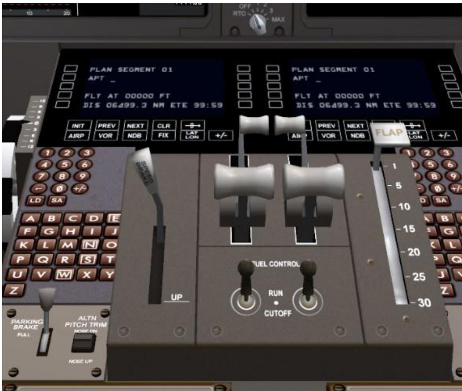
The main controls are the thrust levers, flaps, speed brakes, parking brake, and fuel cut-off levers.
